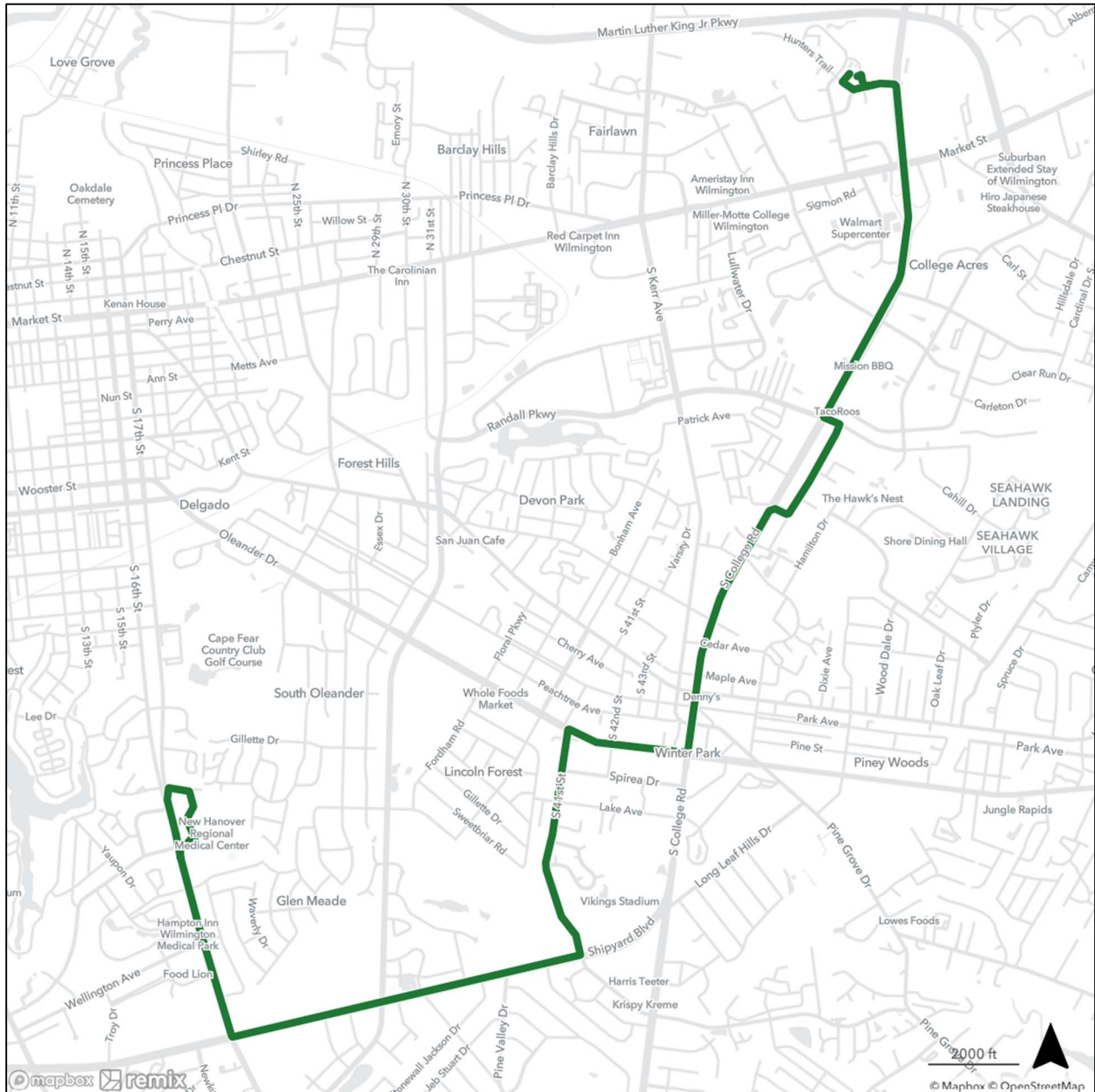
Figure 10 | A redesigned Route 103 could operate between the Medical Center and Forden Station via South 41st St, College Road, and UNCW to provide better effective headways along College Road together with Route 107. Seahawk Shuttle routes could be reconfigured to better serve local trips in the vicinity of Forden Station and UNCW.
